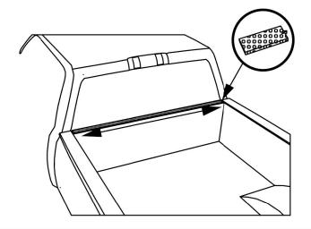
Place Tonneau Cover Assembly on the top of the truck with the straps facing towards the cab window. Unfold the Tonneau Cover to the tailgate and ensure the Tonneau covers the entire top of the truck and is spaced evenly.
