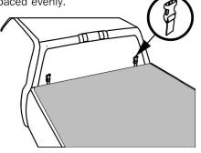
Pull down the Cab & Tailgate Clamps and move the Utility Brackets until the latches line up.
